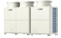
Throughout the year, many buildings require cooling in some areas and heating in others - even in adjacent rooms. The outstanding City Multi R2 system meets this requirement by distributing surplus heat from cooling operations (and vice versa) to rooms where it is needed. This efficiency can result in energy savings of up to 30% over conventional systems.
